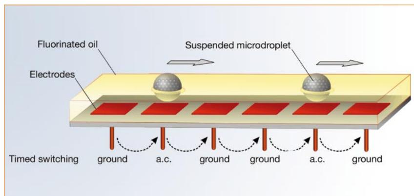
**Figure 1** Schematics of the dielectrophoretic transporter used for the operation of a liquid–liquid microfluidic chip with freely suspended droplets. Water or dodecane droplets of volume 500–1,000 nanolitres float freely on the surface of perfluoromethyldecane ('F-oil', an inert, dense liquid)<sup>13</sup>. Alternating (a.c.) and/or constant electric fields are applied by arrays of electrodes immersed in the F-oil phase a few millimetres below the surface.
