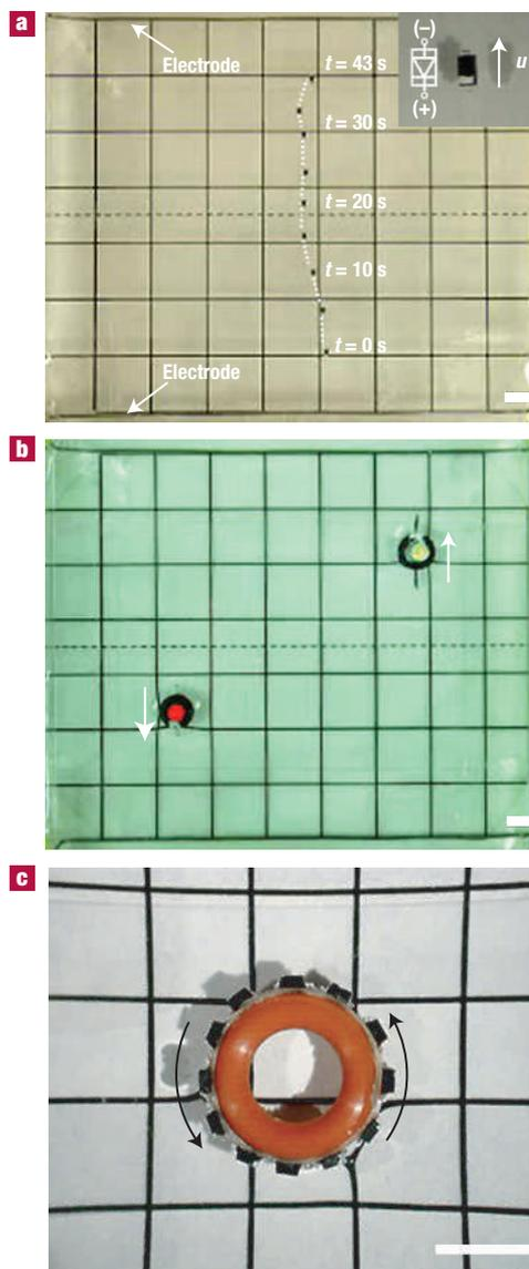
**Figure 2** Optical micrographs of self-propelling semiconductor 'particles'.
