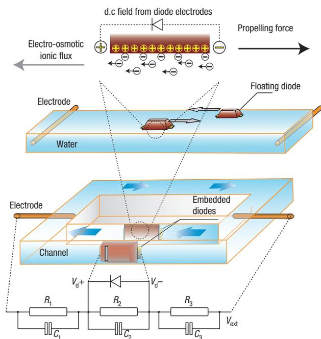
**Figure 1** Schematic diagrams of the experiments for measuring floating-diode velocity and diode pumping rate in a model microfluidic device. The origin of the localized electro-osmotic flow and the equivalent electric circuit used to analyse the magnitude of the d.c. voltage,  $V_d$ , induced in the diode are shown in the top and bottom respectively.
