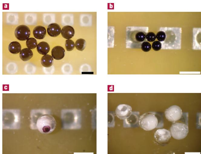
**Figure 4** Polymer-based and polymer-encapsulated particles. **a**, Polymerized SU-8 droplets laced with uniformly dispersed gold nanoparticles. **b**, Solid semiconductive polypyrrole spheres. **c**, Dried 'eyeball' supraparticle encapsulated in polymerized HDDA. **d**, 'Cups' from polymerized HDDA with polystyrene latex deposited inside by drying of the originally encapsulated water droplets. Scale bars, 1 mm.
