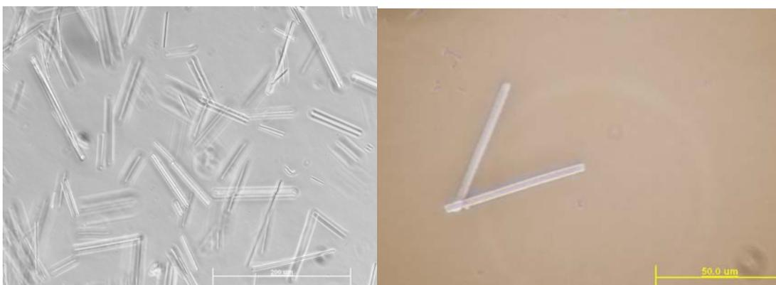
**Figure 4.** Images of SU-8 rods formed in water containing polyvinyl alcohol (PVA). The concentration of PVA allowing rod synthesis has to be in a range in which its water solutions meet the criteria for the viscous ratio and stress. The shear flow is created by a magnetic stirrer.
