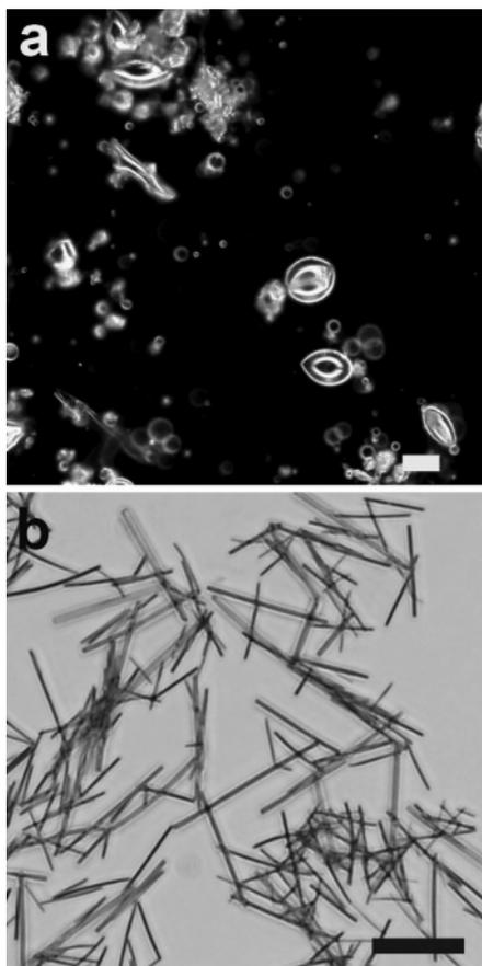
**Figure 8.** Effect of the polymer concentration and viscosity ratio,  $p$ , on the microrod formation process: (a) optical microscopy image of polymer drops solidified when the initial SU-8 solution is emulsified at a viscosity ratio of 0.02; (b) well-shaped rodlike particles at a high viscosity ratio of 0.2. The dispersion medium is glycerin, and the initial concentration of SU-8 is 31 wt %. The scale bars are 50  $\mu\text{m}$ .
