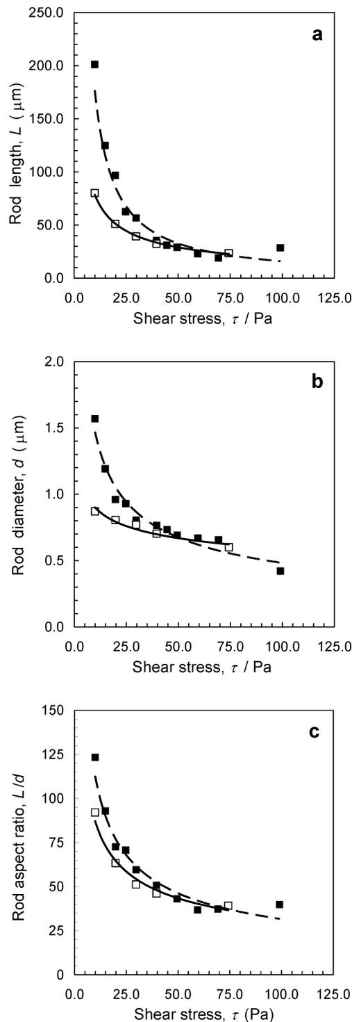
**Figure 5.** Average (a) length, (b) diameter, and (c) aspect ratio,  $L/d$ , of SU-8 rods prepared in 50:50, v/v, glycerol and ethylene glycol as a function of the shear stress. The shear stress is varied through the shear rate. Symbols present data obtained at two different concentrations of SU-8 in the initial polymer solution, 63 wt % (solid symbols) and 48.2 wt % (empty symbols). The lines are a guide to the eye.
