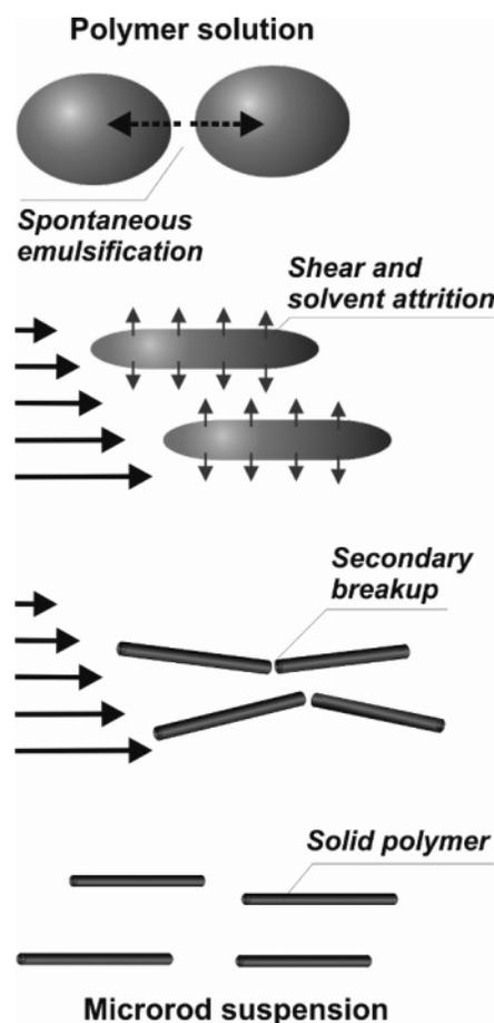
**Figure 4.** Schematics of the stages of the microrod formation process.
