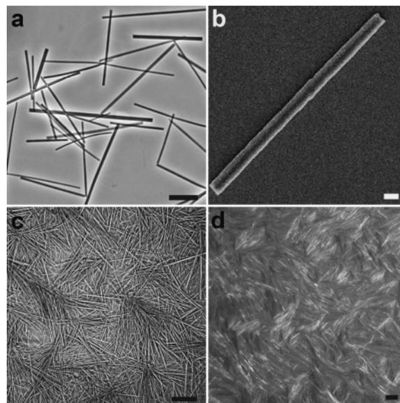
**Figure 1.** Typical optical microscopy (a, c, d) and SEM (b) micrographs of SU-8 rod suspensions with different solid contents. Image c shows a concentrated dispersion of SU-8 rods in water sedimented on the bottom surface. Image d is a micrograph in crossed polarizers of a layer of SU-8 rods deposited on a glass slide after drying of a drop of rod dispersion in dodecane. The scale bar is 10  $\mu\text{m}$  for (a), 1  $\mu\text{m}$  for (b), and 50  $\mu\text{m}$  for (c) and (d).
