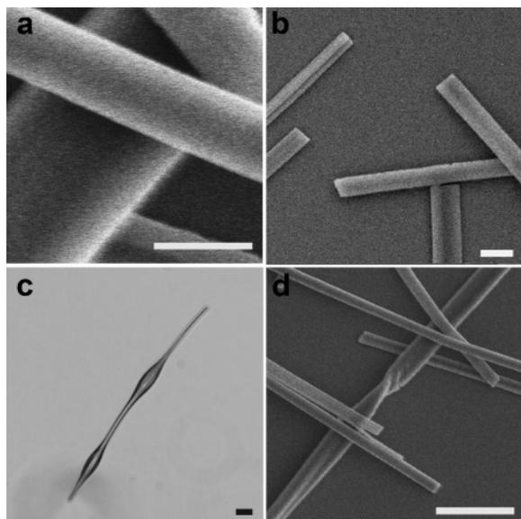
**Figure 2.** SEM (a, b, d) and optical (c) micrographs of SU-8 rods. Frames a and b demonstrate the uniform cylindrical shape and the sharp edges at the ends. Frame c is an intermediate structure solidified at an early stage of the process, and frame d captures a rod solidified in the process of breaking. The scale bar is  $1\ \mu\text{m}$  for (a) and (b) and  $10\ \mu\text{m}$  for (c) and (d).
