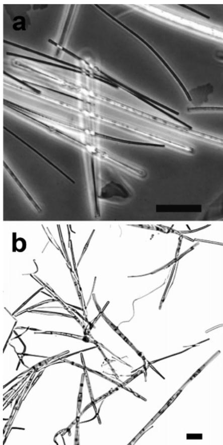
**Figure 9.** Examples of composite rods formed by dispersing inorganic particles in the initial SU-8 solution, which remain trapped within the microrods: (a) rods containing silica spheres and (b) rods containing paramagnetic particles. The scale bars are 10  $\mu\text{m}$ .
