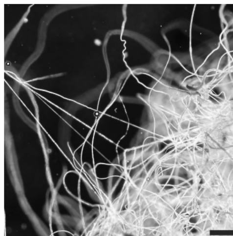
**Figure 3.** Optical low-magnification micrograph of the result of shearing of a solution of polystyrene of high molecular weight. As the polymer threads are flexible and do not break, the final result is long thin polystyrene fibers instead of rods. The scale bar is  $200\ \mu\text{m}$ .
