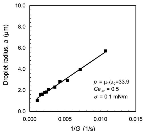
**Figure 7.** Calculated radius,  $a$ , of the hypothetical emulsion drops that would correspond to the final rod size measured. According to the expression for the capillary number, the dependence of  $a$  on the inverse shear rate,  $G^{-1}$ , should be a straight line. The correlation coefficient here is 0.99. Assuming  $\gamma = 0.1$  mN/m, the critical capillary number calculated from the slope is  $Ca_{cr} = 0.5$ .
