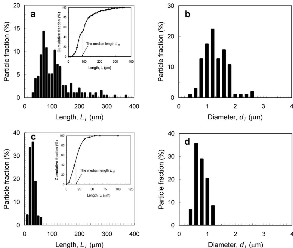
**Figure 6.** Particle length (a, c) and diameter (b, d) distribution (by number) for rods synthesized at (a, b) a low shear stress of 14.9 Pa and (c, d) a high shear stress of 59.4 Pa. The dispersion medium is glycerol/ethylene glycol at a 1:1 volume ratio.
