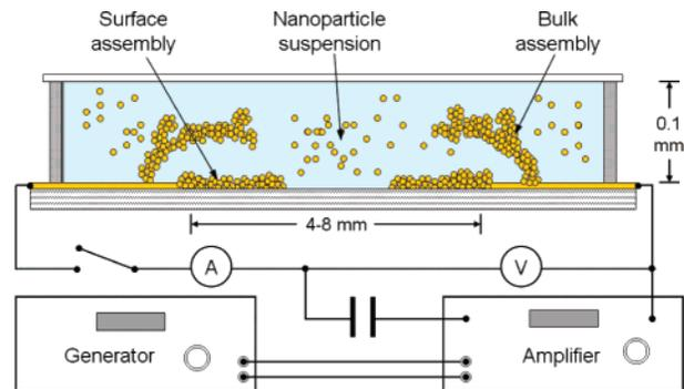
**Figure 1.** Outline of the experimental setup and schematics of the two different modes of microwire growth—bulk microwire assembly and surface microwire assembly. The chamber and the nanoparticle sizes are not to scale.
