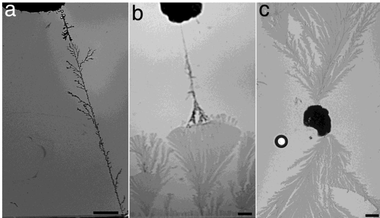
**Figure 9.** Various types of microwire electrical connections to conductive islands between the electrodes. Islands connected through (a) bulk microwire growth only, (b) a combination of bulk and surface growth, or (c) surface assembly only. Scale bars: 500  $\mu\text{m}$ .
