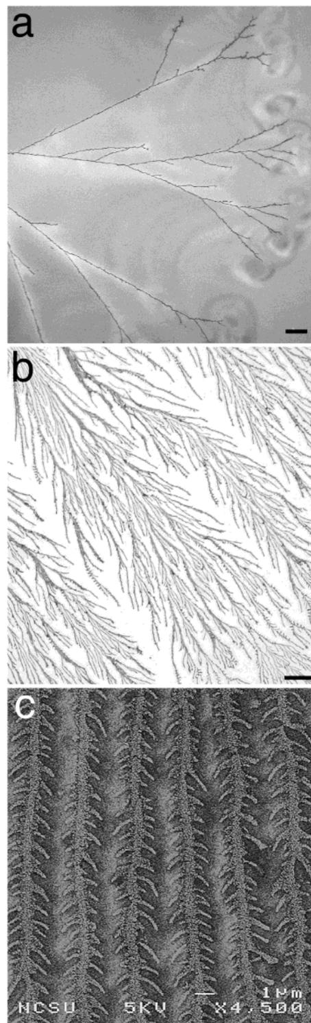
**Figure 2.** Typical experimental images of the two types of microwire structures obtained. (a) Bulk microwire growth. Note that some of the branches are not in the focal plane. (b) Surface microwires. (c) Scanning electron micrograph of the surface microwire structure. Scale bars: (a) 100  $\mu\text{m}$ ; (b) 20  $\mu\text{m}$ .
