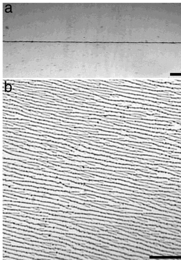
**Figure 8.** Controlled assembly of microwires with a specific morphology: (a) single unbranched microwire grown through the bulk nanoparticle suspension containing 50% glycerol by volume; (b) array of parallel wires assembled on the surface of a glass slide. Scale bars: 50  $\mu\text{m}$ .
