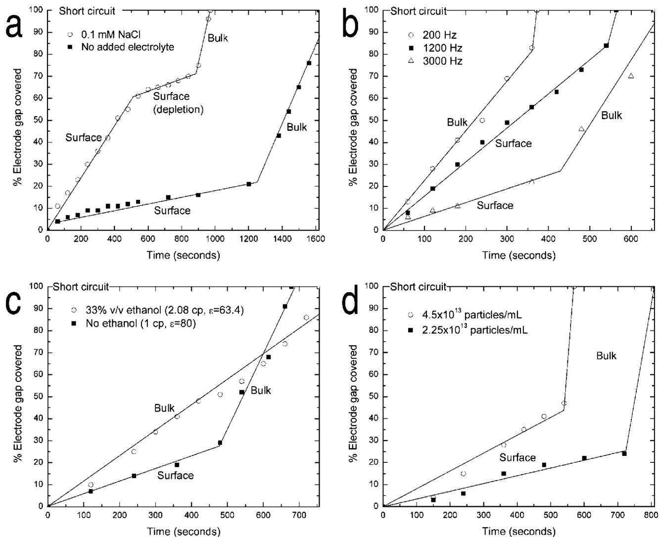
**Figure 4.** Effect of the operating parameters on the assembly speed of microwires: (a) electrolyte; (b) frequency; (c) viscosity and dielectric constant of the medium; (d) particle concentration. In all experiments the other parameters were kept constant. Note that in all plots the growth speed for bulk assembly is higher than that for surface assembly. Solid lines are guides to the eye.
