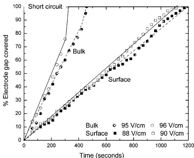
**Figure 3.** Speed of microwire assembly in bulk and surface modes plotted as percentage of electrode gap covered versus time. Two microwires were grown in each assembly mode to evaluate the reproducibility of the process. Lines are guides to the eye.
