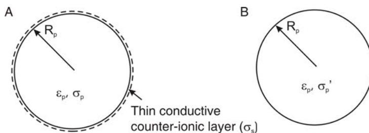
**Figure S2.** Models of latex microspheres in aqueous media: **(A)** Thin conductive counter-ionic layer surrounding the latex microsphere. **(B)** Simplified structure with effective polarizability equivalent to the shell type structure in (A).
