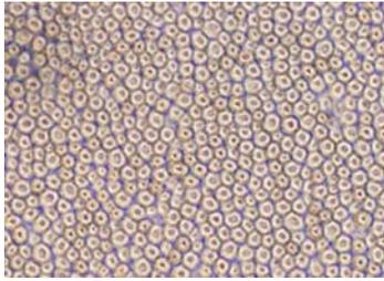
**Movie 5: 2D array formation of cells using 4-point electrodes.** Yeast cells (0.08 % w/v) aligned alternatively in two orthogonal directions using an AC electric field of 75 V and 30 Hz in the four-electrode chip. The cells assemble into 2D arrays. The movie was taken over 30 min at 1 frame min<sup>-1</sup>.
