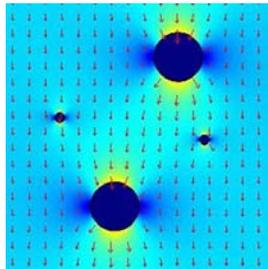
**Movie 4: Numerical simulation of a two cell – two particle co-assembly process.** 2D electrostatic computation of dynamic assembly of yeast cells and  $1 \mu\text{m}$  latex spheres in DI water performed using FEMLAB. The electric field distribution and effective polarizabilities show how one of the latex microspheres gets entrapped between the cells due to positive dielectrophoresis.
