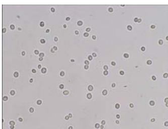
**Movie 1: Electric field directed assembly of cells into chains.** AC electric field of  $13 \text{ V mm}^{-1}$  and 100 Hz between two parallel coplanar electrodes applied across a suspension of 0.01 % w/v *S. cerevisiae* yeast cells in PBS. The cells align into chains parallel to the electric field. This movie has been speeded up 40 $\times$ .
