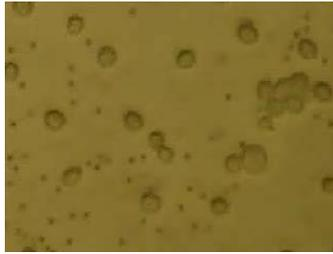
**Movie 3: Experimentally observed co-assembly of yeast cells and latex particles.** AC electric field of  $10 \text{ V mm}^{-1}$  and 30 Hz between two parallel coplanar electrodes applied across a mixture of 0.1 % w/v yeast cells and 0.1 % w/v  $1 \mu\text{m}$  sulfate stabilized latex microspheres in DI water. The cells and particles align alternatively along the field direction. This movie has been speeded up  $8\times$ .
