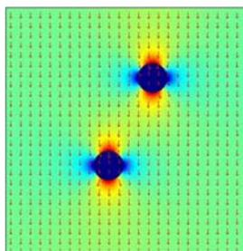
**Movie 2: Numerical simulation of cell chain assembly in electric field.** 2D electrostatic computation of effective yeast cell polarizability in PBS performed using FEMLAB. The electric field distribution around the cells illustrates how cells arrange into chains collinear to the applied field due to positive dielectrophoresis.
