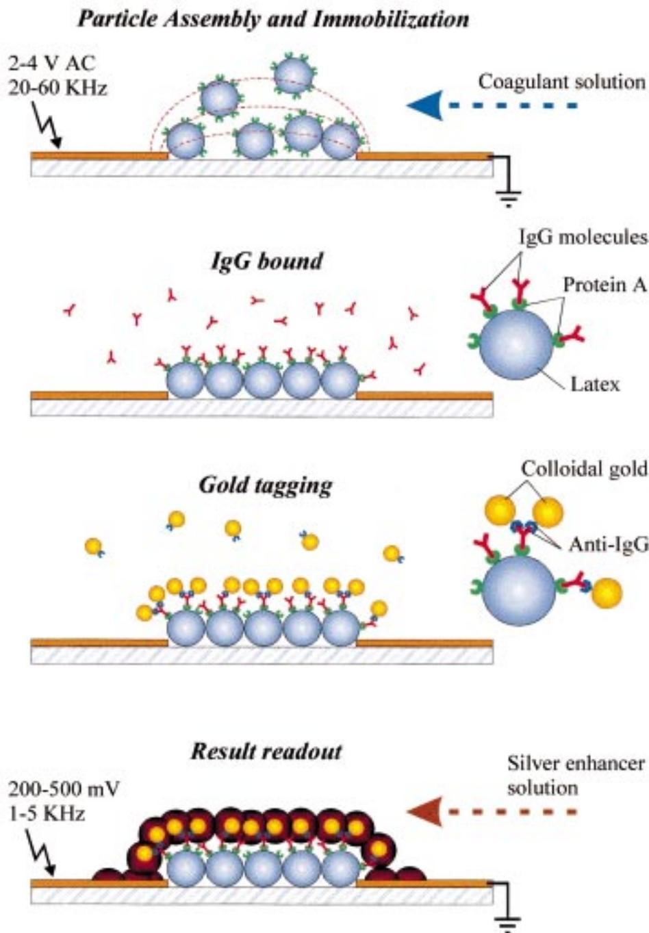
**Figure 1.** Schematics of the main stages of sensor assembly and functioning. The procedure is illustrated by an immunoglobulin test.
