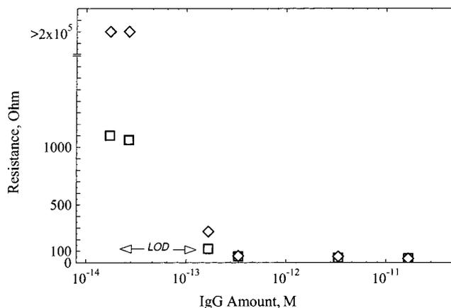
**Figure 4.** Sensor resistance as a function of the IgG amount. The squares and diamonds at each concentration show the results of two different experimental runs. The two points above the scale break denote an open circuit (resistance higher than the multimeter range).
