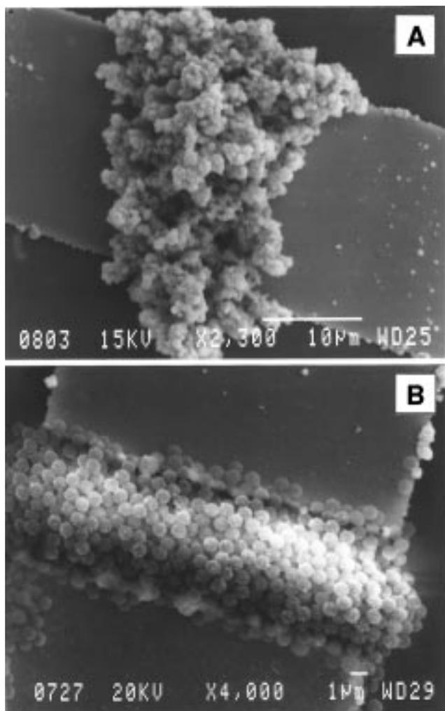
**Figure 3.** SEM micrographs of gold-tagged and silver-enhanced latex bridges between electrodes in IgG-specific experiments. (A) Protein A-functionalized latexes heavily coated by deposited metal that short-circuits the electrodes. (B) Nonfunctionalized particles in the negative control patches only marginally tagged by deposited metal. The bridge remains nonconductive.
