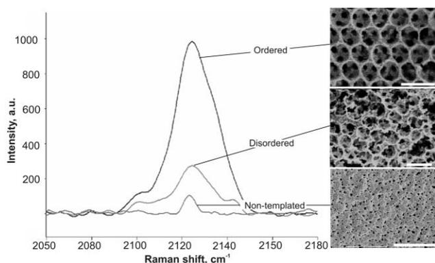
**Fig. 2** Effect of substrate structure on the SERS signal intensity. Characteristic sodium cyanide spectra and SEM images collected in the continuous sampling microfluidic flow cell for ordered latex-templated (top), disordered latex-templated (middle), and non-templated (bottom) SERS substrates. Scale bars are 1  $\mu\text{m}$  (top and middle micrographs) and 10  $\mu\text{m}$  (bottom micrograph).<sup>19</sup>
