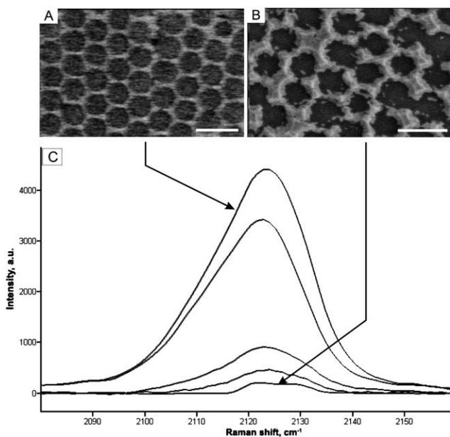
**Fig. 3** Effect of the substrate nanoporosity on SERS spectra intensity. SEM images collected from the (A) non-fused and (B) fused regions of the substrate with a nanoporosity gradient. Scale bars = 1 μm. (C) Raman spectra collected sequentially moving from the non-fused end (top spectra) to the highly-fused end (bottom spectra).<sup>19</sup>
