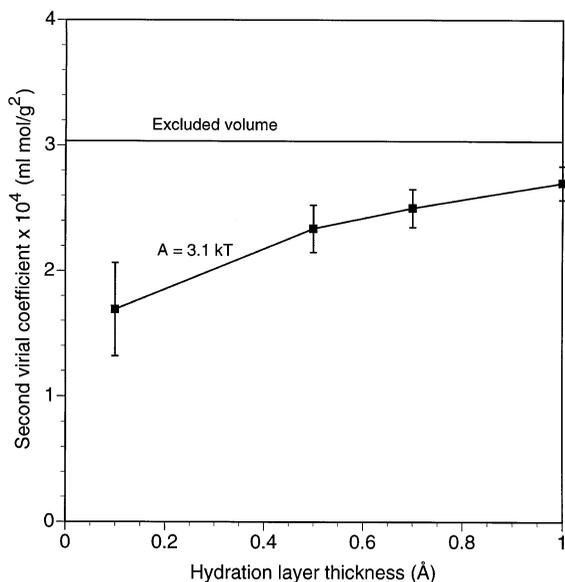
Fig. 5. Calculated values of second virial coefficient based on crystallographic structure of chymotrypsinogen, shown as a function of hydration layer thickness. Only excluded volume and van der Waals interactions are included.
