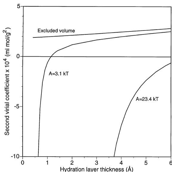
Fig. 4. Calculated values of second virial coefficient for sphere model, showing dependence on value of hydration layer thickness and Hamaker constant. Only excluded volume and van der Waals interactions are included.
