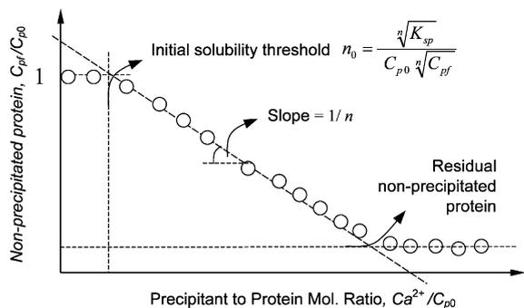
Fig. 1. Explanation of the model used for interpretation of precipitation data.
