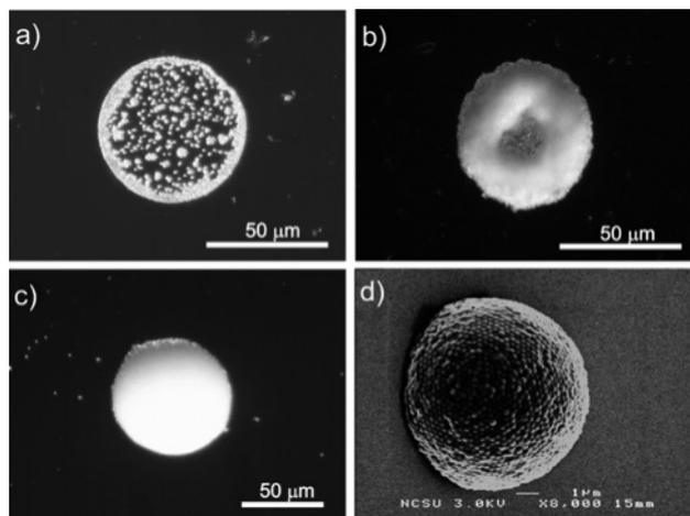
**Figure 1.** Micrographs of micropatches deposited from sessile droplets of 600 nm latex particle suspension on (a) hydrophilic glass, (b) hydrophobic silane-treated glass with latex particle concentration  $<1$  wt %, and (c) same substrate at a particle concentration  $>1$  wt %. (d) SEM image of a hemispherical assembly similar to that shown in (c), imaged at a tilt angle of  $30^\circ$ .
