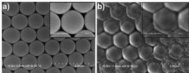
**Figure 3.** SEM micrographs showing the microstructure of hemispherical assemblies comprised of 910 nm microspheres (a) as-deposited, and (b) sintered for 5 min at 110 °C. Note the slight deformation of the partially fused particles in (b).
